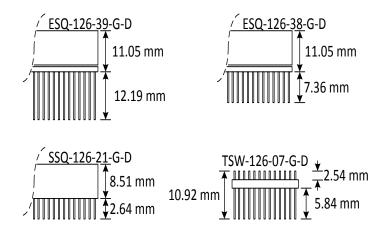
**Note:** The middle reference point is the top of the board. The iOBC board is 1.7mm thick.
