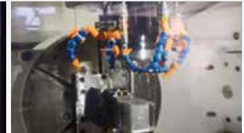
4. Machining by 5-axis MC 1U MBF is completed in 24 hrs.
