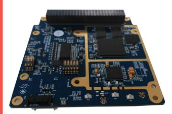
**TOTEM-UHF-Frontend** is a **UHF front end piggyback board**, with maximum output power of 30 dBm. It also behaves as an **antenna switch**, allowing you to share the UHF antenna with up to 2 more devices.
